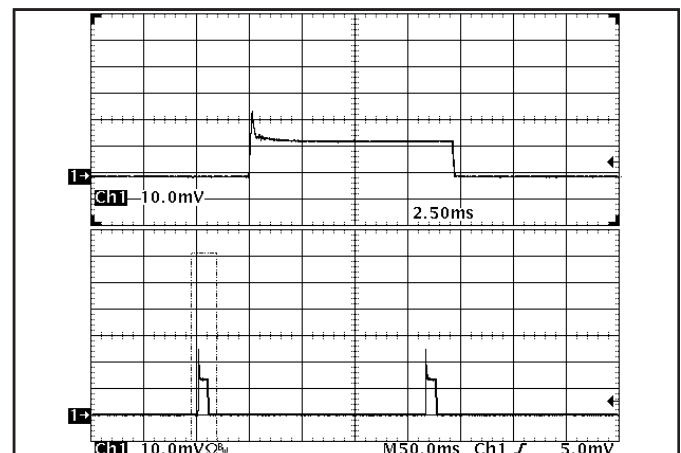
Figure 18: Load current ( 10\ \text{A}/\text{div} ) as a function of time when the converter attempts to turn on into a 1\ \text{m}\Omega short circuit. Top trace ( 2.5\ \text{ms}/\text{div} ) is an expansion of the on-time portion of the bottom trace.
